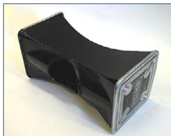
The Hush-a-Phone, a noise-reduction device used in early SI systems
